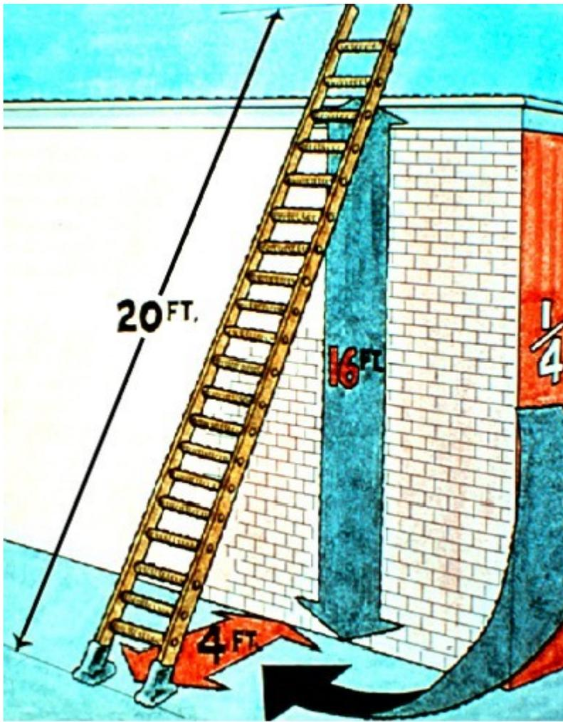
The photo below shows how a worker in the field can quickly verify that their extension ladder is at a safe angle.
